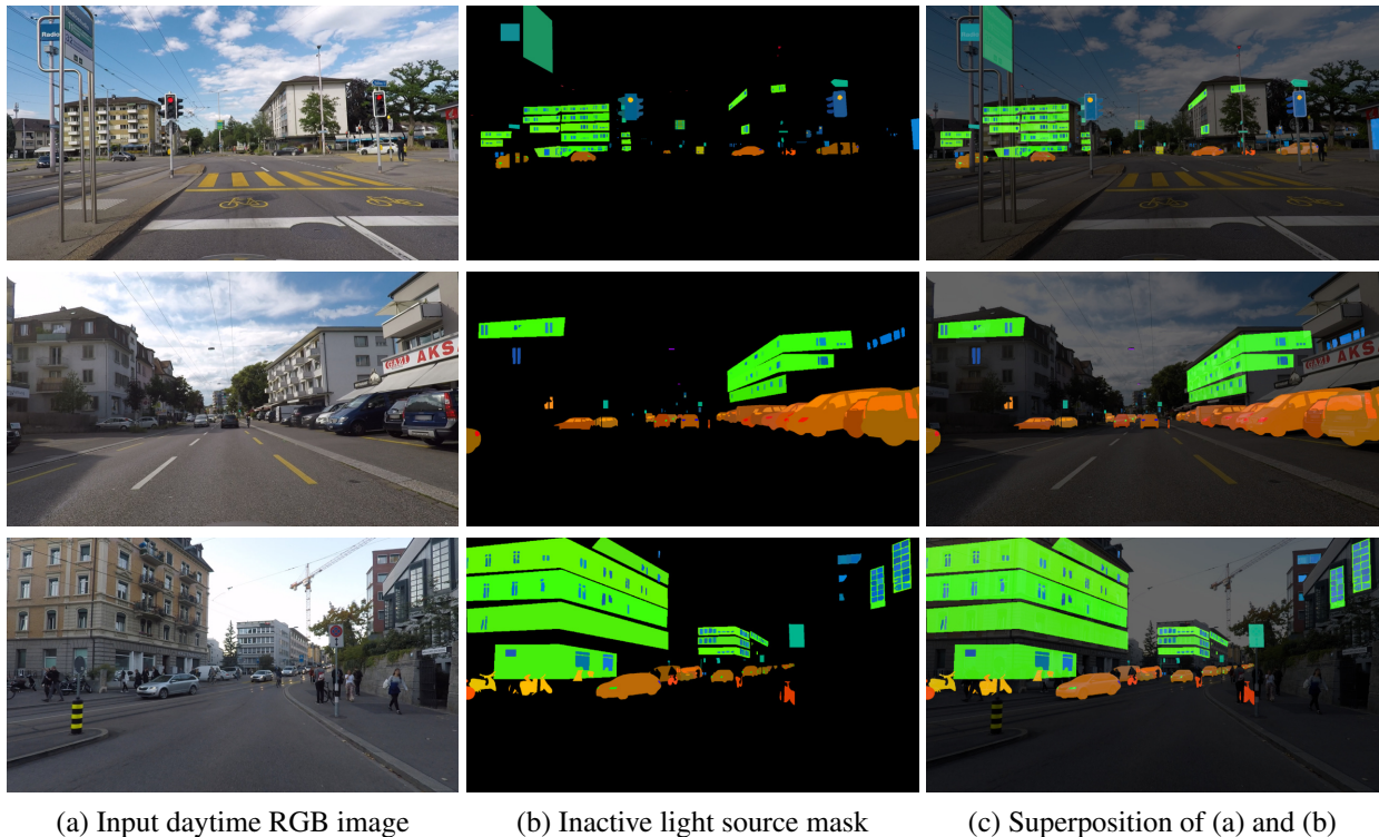
Figure 3.3: Annotation Examples. We present several examples of our inactive light source annotation. The left column shows the input daytime RGB image, the middle column shows the annotated inactive light source mask, where each instance has its own identity and bounding box, and the right column superimposes the RGB image and the light source mask.
