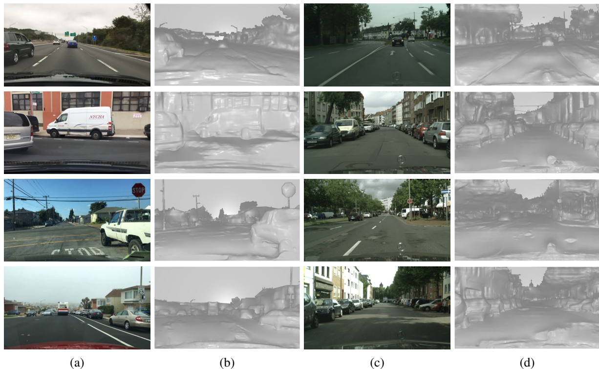
Figure 4.5: Mesh reconstructed from different datasets. We showcase the mesh reconstruction based on two different datasets: BDD100K dataset [65] (column (a) and (b)) and Cityscapes dataset [6] (column (c) and (d)). The above results demonstrate the capability of our pipeline to generate reasonable scene mesh when applied to other datasets. However, we notice that roads close to the camera are not correctly reconstructed, this is a result of inaccurate surface normal prediction caused by the ego vehicle.
